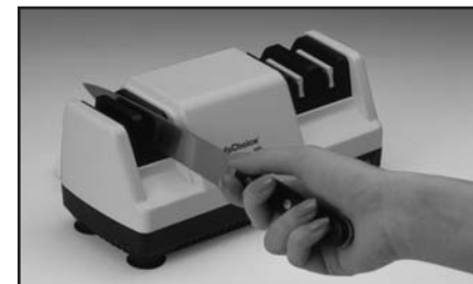
Stage 1— Three (3) or more* slow passes through each slot, (left and right PRE-SHARPENING slot). Alternate each pass.
